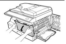
Gently pull the TD (Toner/Developer) cartridge out while pressing the lock release button.
